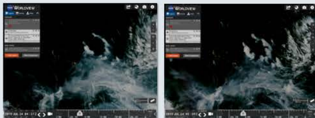
Above: in this arctic fire example, the image on the right was acquired approximately 90 minutes after the image on the left; during that time, the smoke and fire locations have visibly changed; those changes would be impossible to see if the swaths were mosaicked into a single image.
