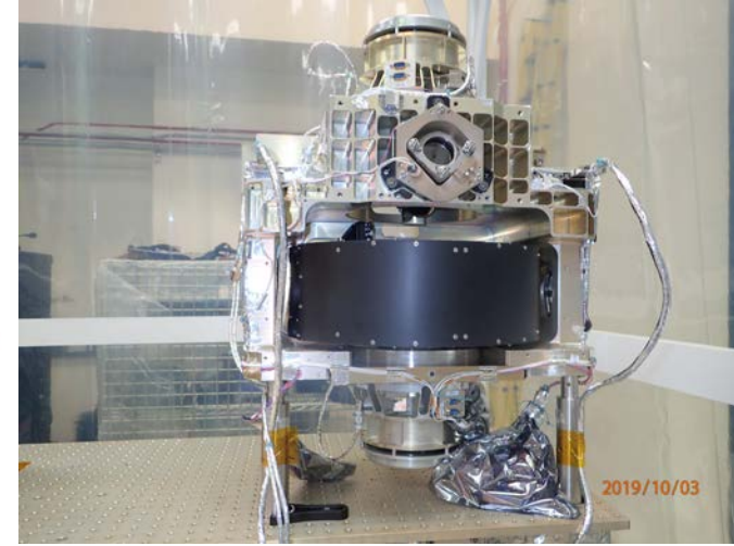
OCI ETU FlatSat End-to-End Electrical System Test
