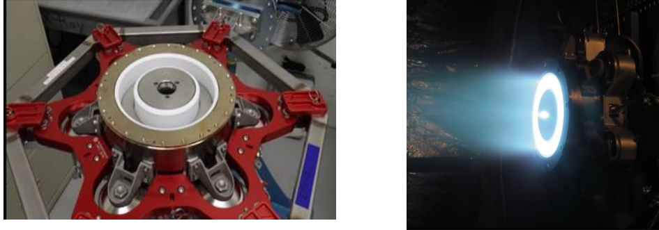
Figure 11 – AEPS ETU-1 Thruster in Assembly and in Hot Fire Testing at JPL
