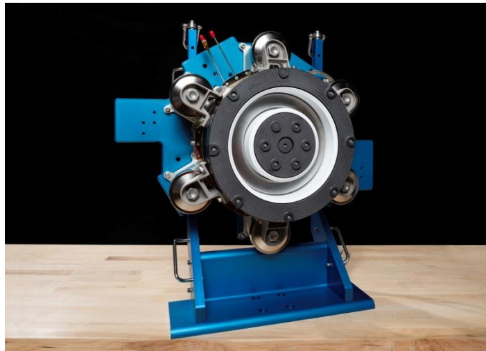
Figure 18. AEPS ETU-1 Hall Current Thruster prior to Integration for Hot Fire Test
