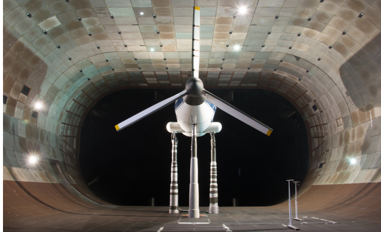
Fig. 1. TTR/699 installed in the NFAC 40- by 80-ft test section, 0-deg yaw.
