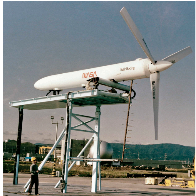
Fig. 4. Scaled JVX rotor on the Prop Test Rig at the OARF (1984).
