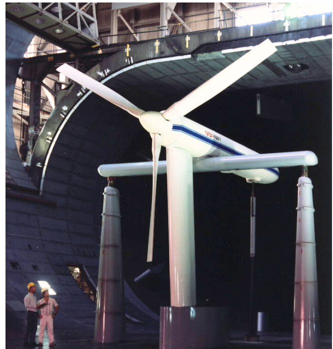
Fig. 5. Scaled JVX rotor on the Prop Test Rig in the NFAC (1991).
