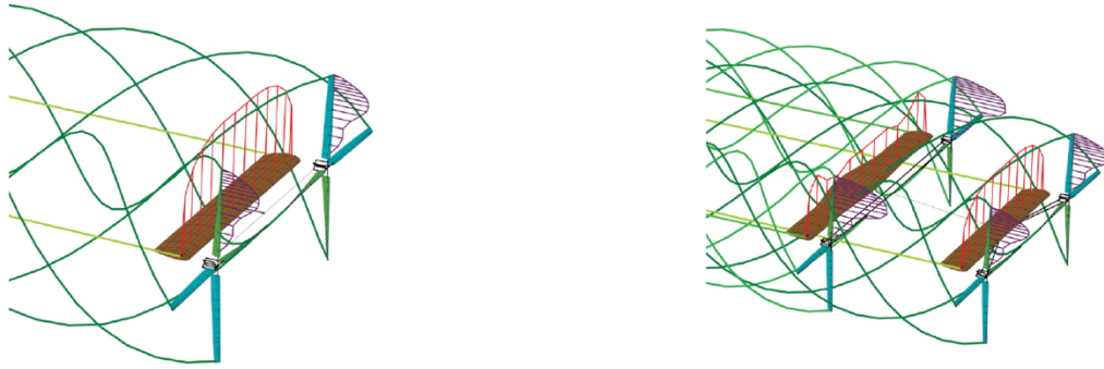
Figure 2.32. Wake geometry of conventional tiltrotor and quad tiltrotor (Figs. 21 (left) and 22 (right) of Johnson et al. [2007]).
