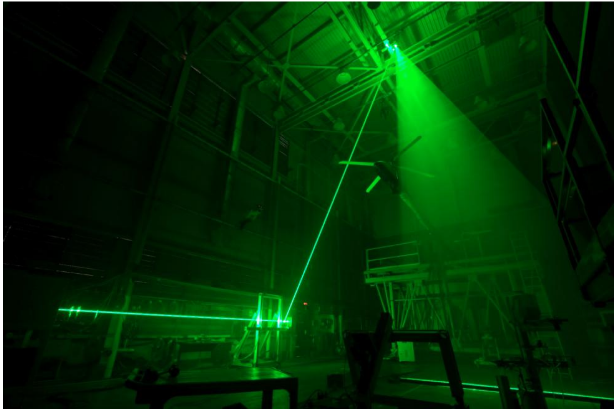
Figure 4.3. PIV laser beam path and light sheet location in the RTC (Fig. 5 of Wong et al. [2010]).
