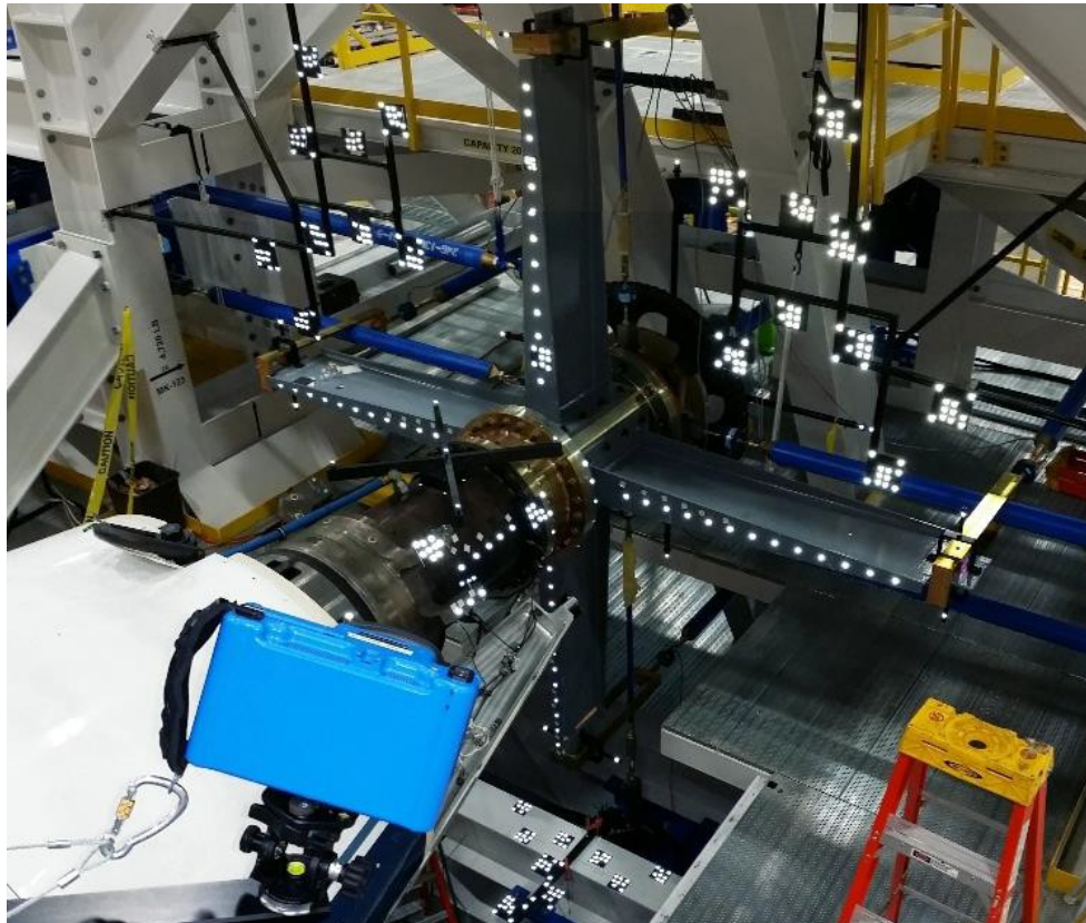
Figure 4.10. Retro-reflective targets installed on deflection hardware and calibration body (Fig. 16 of Solis and Meyn [2016]).
