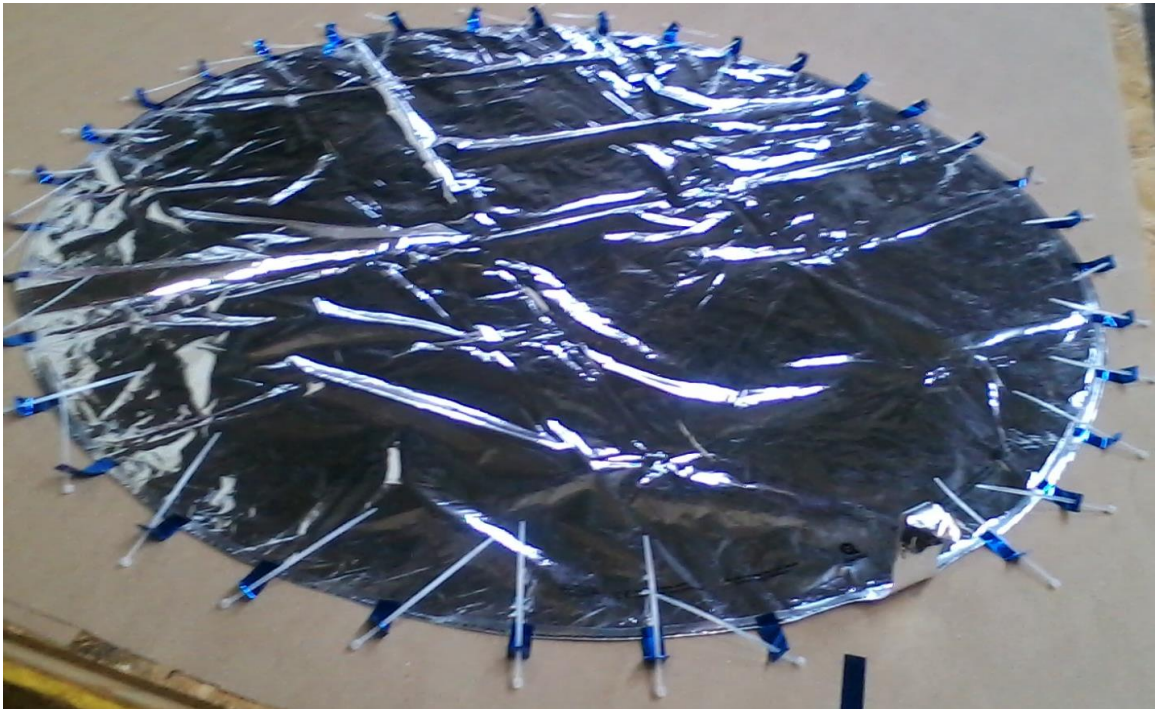
FIGURE 14: Pre-Mounted Inflatable Test Article
