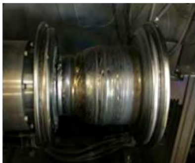
Figure 22. Structural Inconel 625 jacket EBF3 deposited on to SLM Cu liner. Image credit: NASA.
