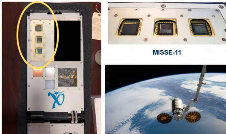
Figure 3. 3D photovoltaic cells made from CNTs on MISSE 11. Image credit: Georgia Institute of Technology.
