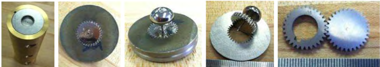
Figure 33. Images of BMG gears made with direct casting. BMG gears have excellent performance at cryogenic temperatures. Image credit: NASA JPL.
