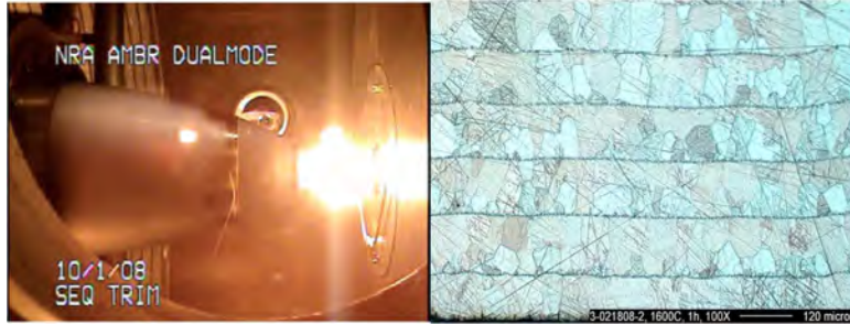
Figure 9. (left) Hot-fire testing of Advanced Material Bipropellant Rocket (AMBR) engine produced by Plasma and Aerojet. (right) Engineered Re structure after annealing at 1,600 °C for 1 hr. Pinning layers have prevented grain growth between the ductile rhenium layers. Image credit: Plasma Processes.
