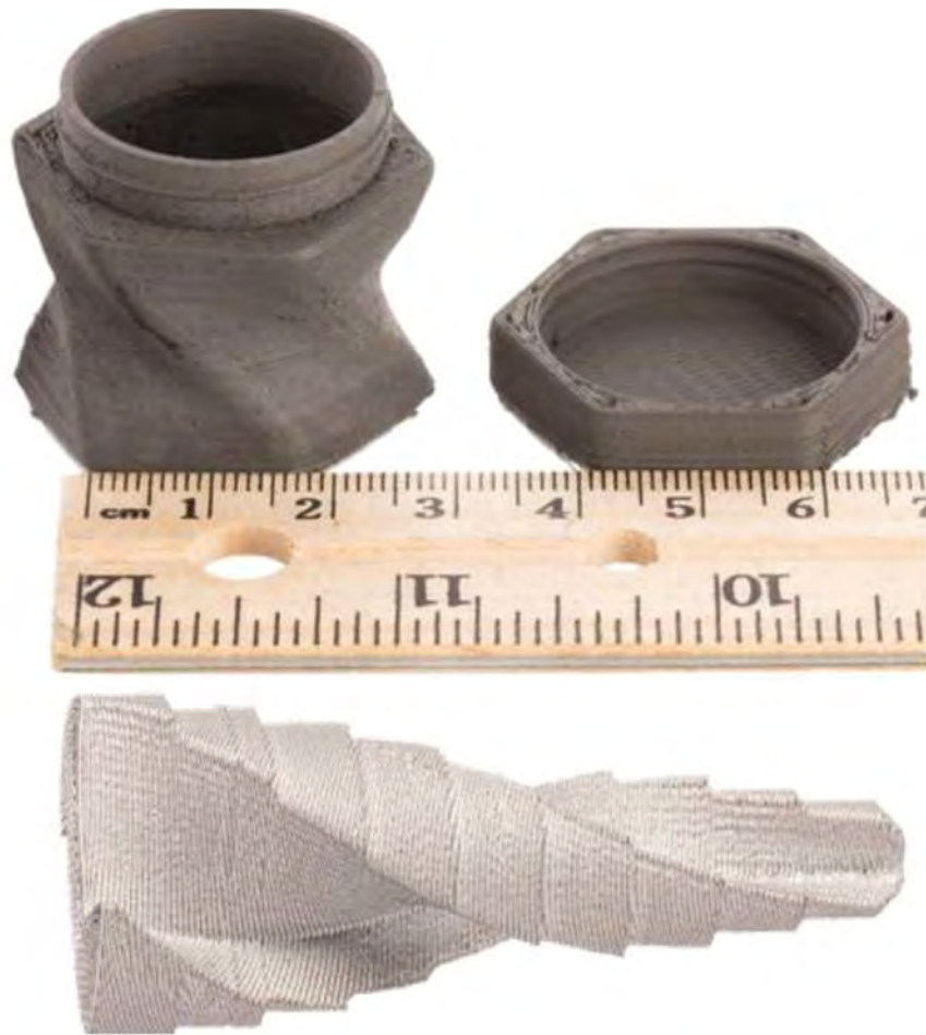
Figure 6. Jar with threaded cap (top image)—shows functionality immediately after sintering. Hollow core geometrically lightweighted step drill bit (bottom image). Image credit: Massachusetts Institute of Technology.
