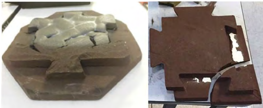
Figure 28. Example of sintered basalt for a paver application. Image credit: Rob Kelso.
