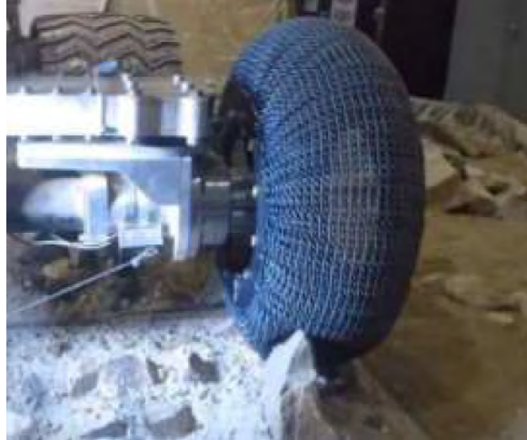
Figure 23. Nickel Titanium alloy spring for rover wheels. Image credit: NASA.
