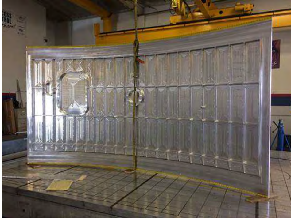
Figure 8. Airware 2050 panel machined and formed in T34 temper and aged to T84 temper. Image credit: Michael Niedzinski, Constellium.
