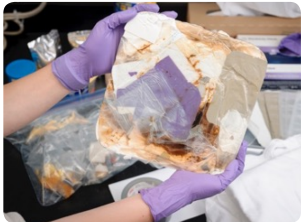
A sample trash tile, compressed to less than one-eighth of the original trash volume, was produced by the Heat Melt Compactor. (Image credit: NASA / Dominic Hart)
