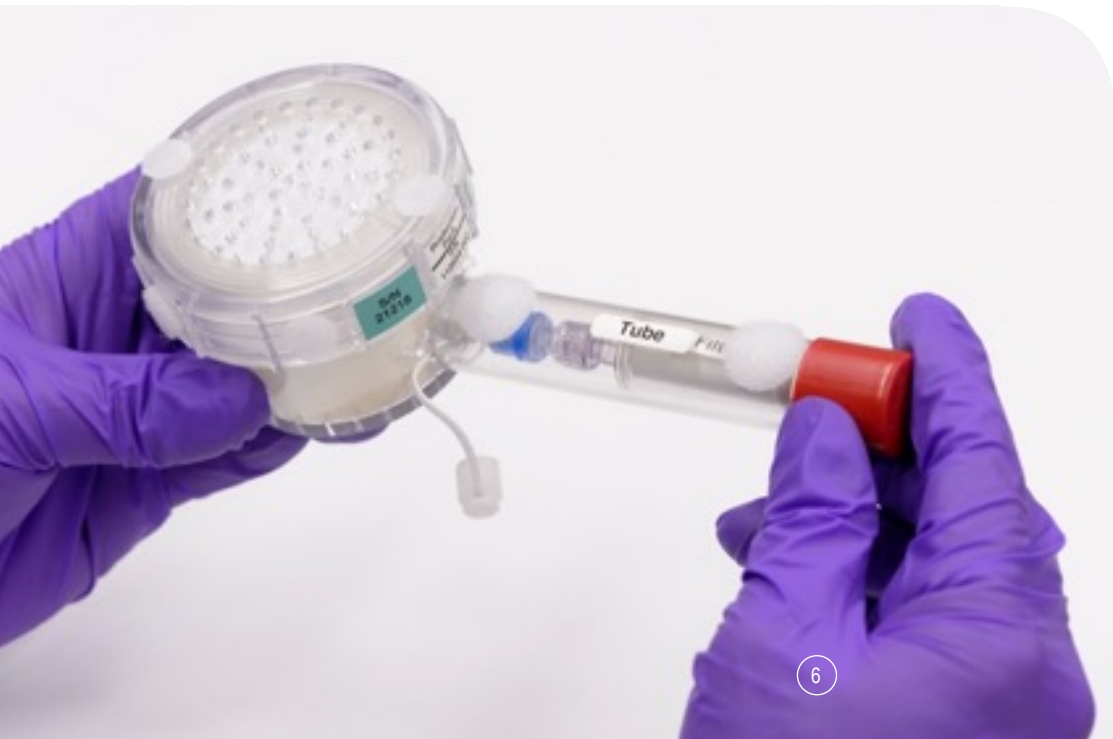
For the BioNutrients experiment, the specially engineered yeast and its powdered food source are held in the container at the left. Its lid holds a membrane that allows carbon dioxide from the yeast to escape. The clear tube at right protects another filter system leading into the compartment with the microorganisms. To activate the yeast and begin the experiment, astronauts on board the space station will inject water through the filter, making it sterile. The water will dissolve the nutrient powder and the yeast will grow and multiply in this liquid environment, producing an important nutrient for human health. (Image credit: NASA / Dominic Hart)
