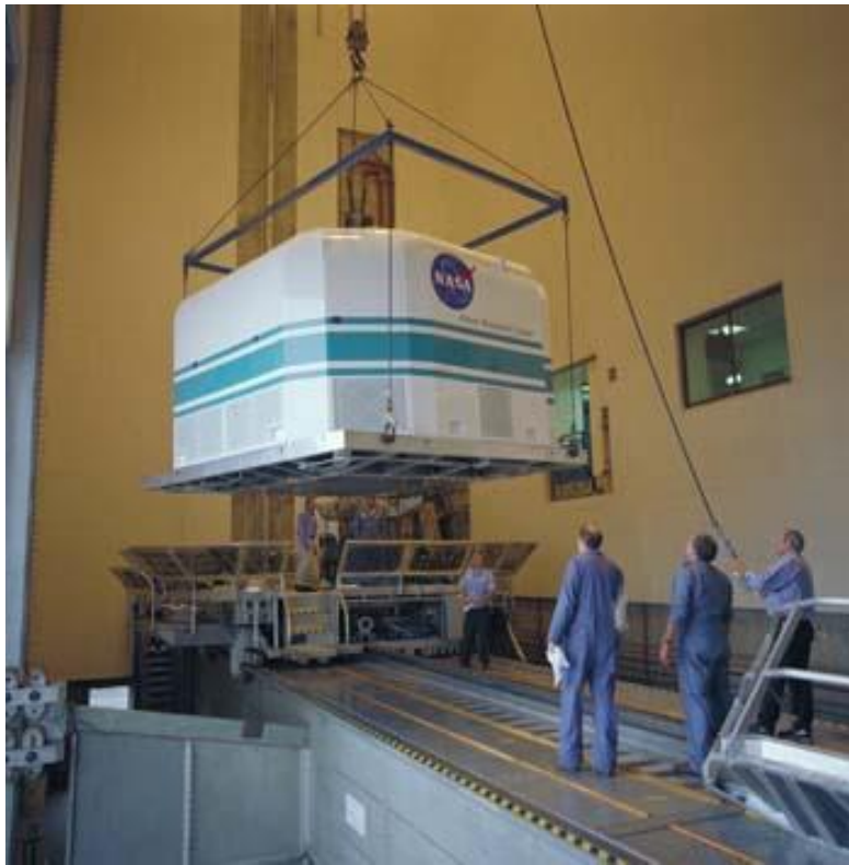
Figure: I-Cab Installation
