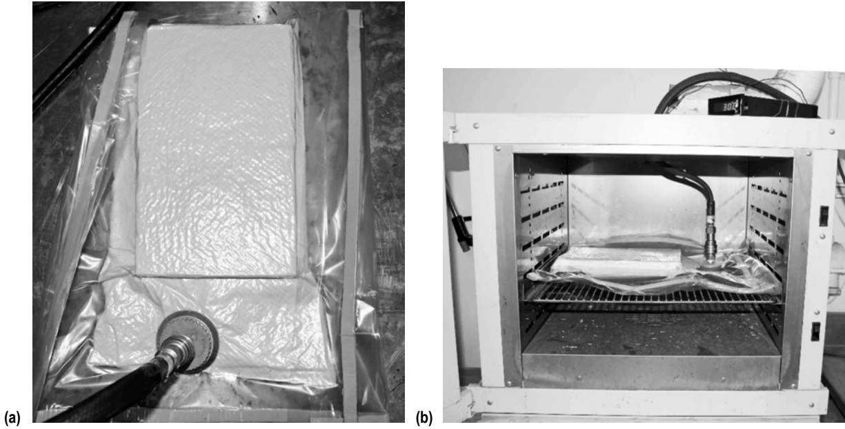
Figure 8. Photographs showing vacuum bagged: (a) repaired specimen and (b) specimen in oven to be cured.
