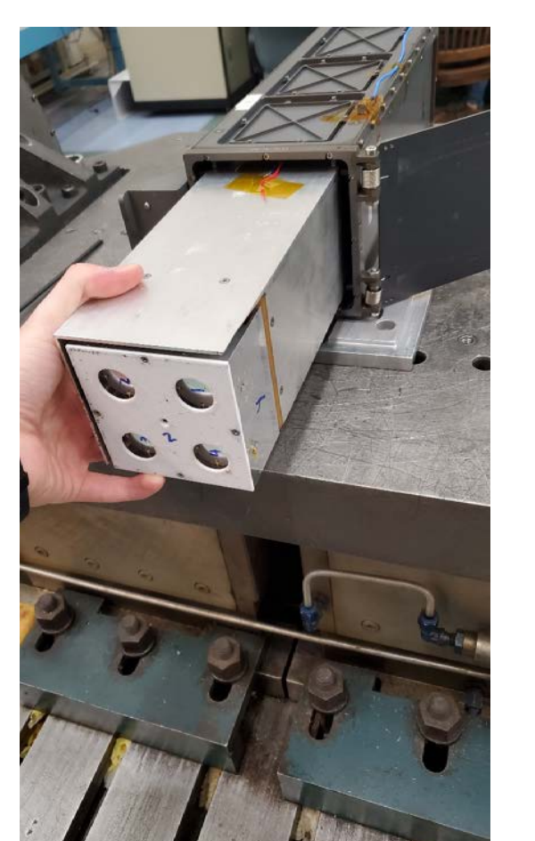
CubeSat prototype fitting inside a PPOD launcher atop the vibration table
