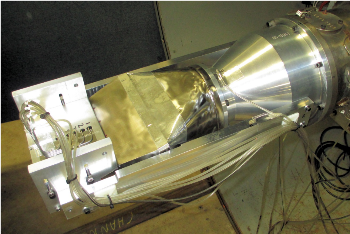
Config 1 - Baseline: NASA one-sided ejector nozzle system.
