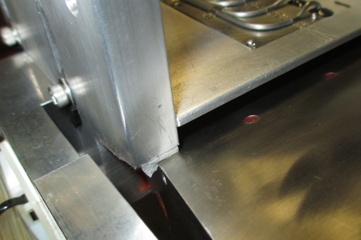
Foam sealing tape used to fill gaps between box side walls and nozzle surface.
