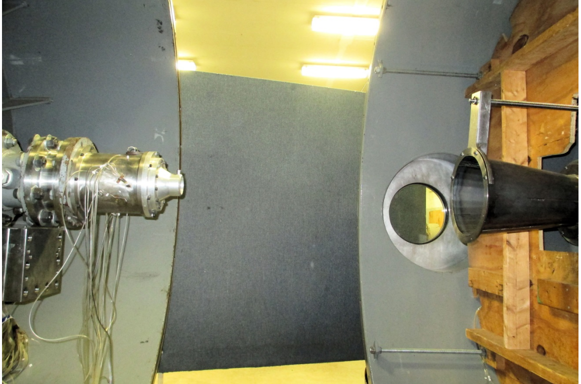
2.25" ASME nozzle assembly, conical collector and 6 inch diffuser. (Test cabin was in the open position for all tests.)
