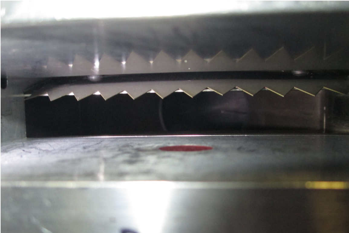
Config 2 – Tab Strip: view inside ejector box of serrated tab strip.
