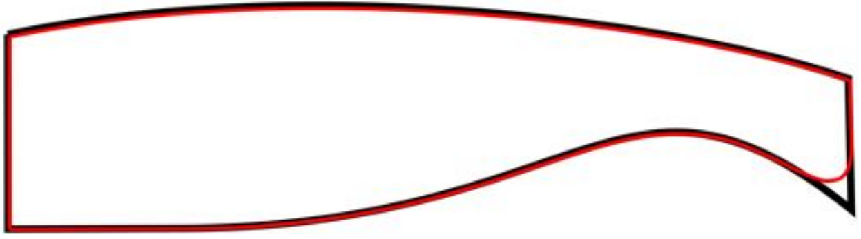
Fig. 40 Illustration of the rounding of the divergent trailing edge. The black curve represents a portion of the divergent trailing edge. The red represents this trailing edge after it has been rounded.
