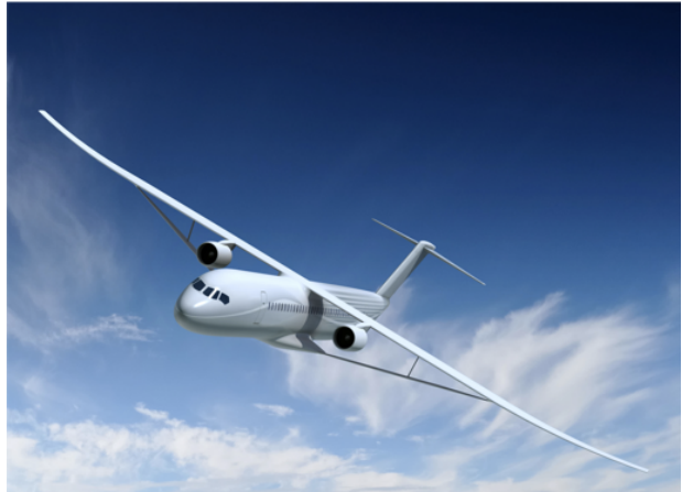
Fig. 1 Rendering of a transonic truss-braced wing model. (Courtesy of Boeing)
