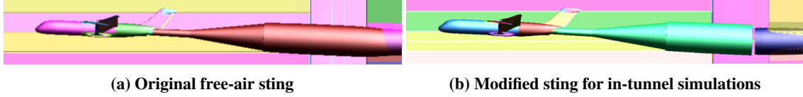
Fig. 21 Modification of TTBW sting geometry to remove overlap and allow rotation of TTBW grid.
