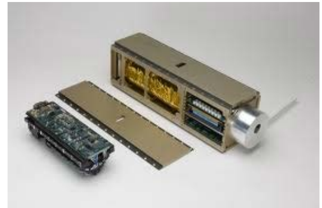
An exploded view of the PharmaSat spacecraft
