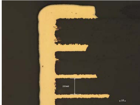
Dielectric layer less than 3.0 mil
