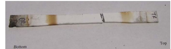
Failed in gage section after 48 hours (1,200 cycles)
