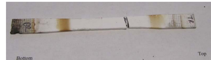
Failed in gage section after 48 hours (1,200 cycles)
