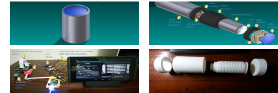
Figure 4 (Top Left) Overview of Preliminary Germination Module, (Top Right) Components view of Germination Module, (Left Bottom) Basic telemetry unit with Android, Arduino, Raspberry Pi, and corresponding sensors, and (Right Bottom) Component view of 3D small sealed module print.
