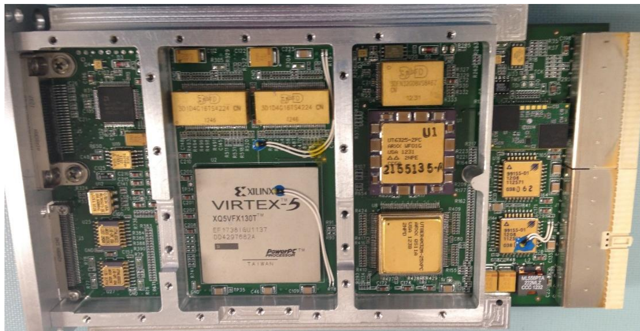
Back-to-Back FPGA Design
