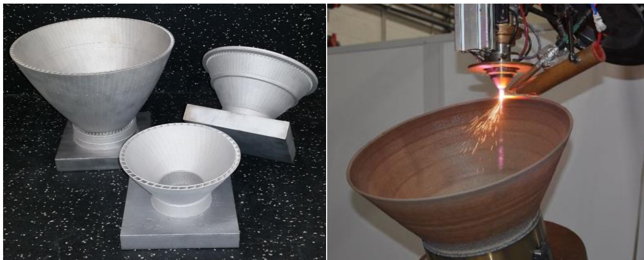
Fig. 11: Examples of integral-channel nozzles and thick-wall mid-scale nozzle, DED NASA HR-1.
