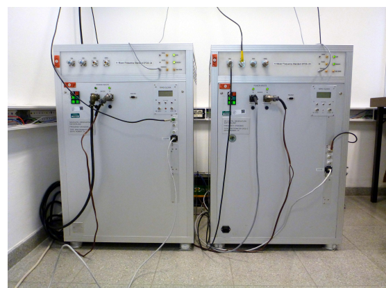
Fig. 6 VLBI reference H-maser EFOS-24 and EFOS-20 at the time & frequency laboratory of AGGO.
