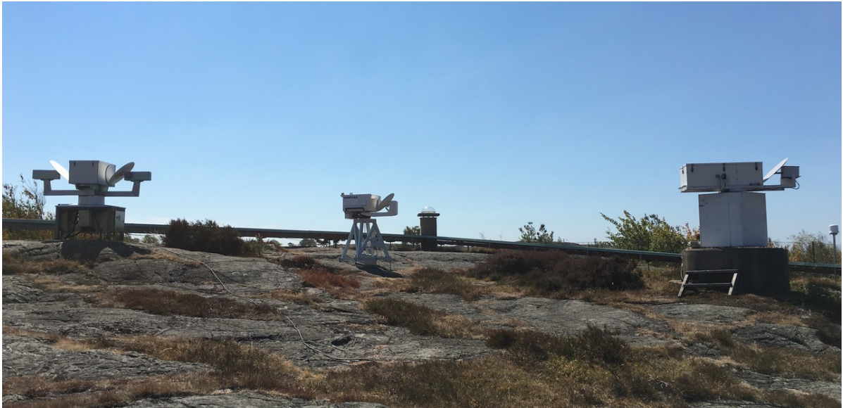
Fig. 4 The three WVRs on the 13th of July 2018. Seen from the left to the right are: Konrad, Orwvar, and Astrid. The main GNSS station ONSA is also seen, just to the right of Orwvar.
