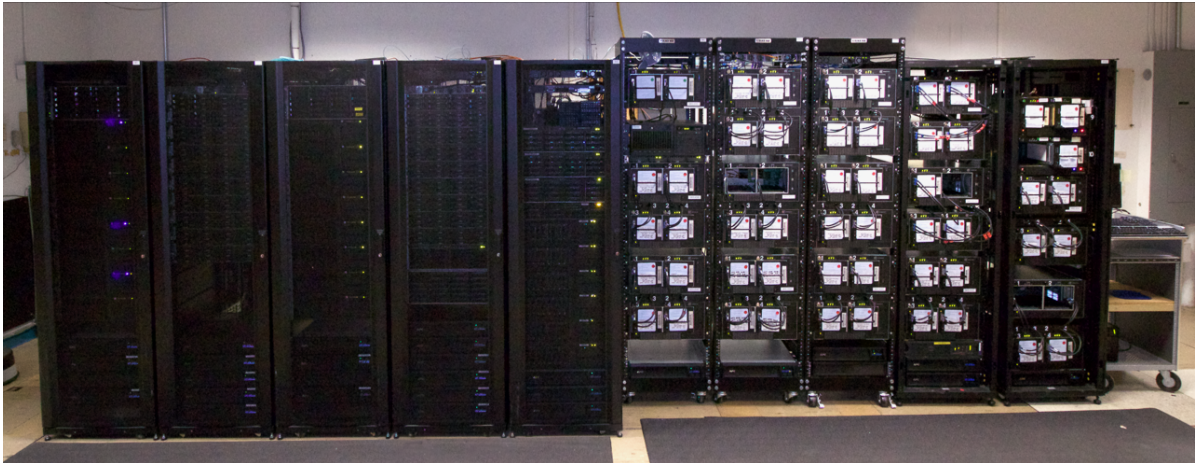
Fig. 1 (Left) Cluster correlator and (right) Mark6 playback units at the MIT Haystack Observatory.
