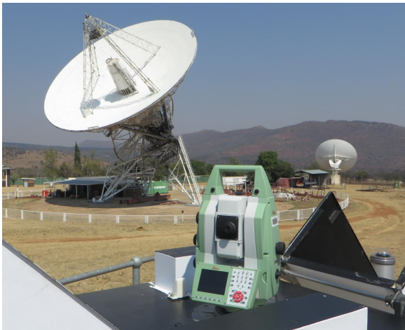
Fig. 5 Leica MS50 Total Station—the local automated site tie system under test with measurements and calibrations being carried out.
