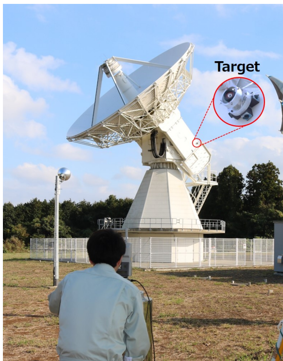
Fig. 3 Picture of field co-location survey by outside method.
