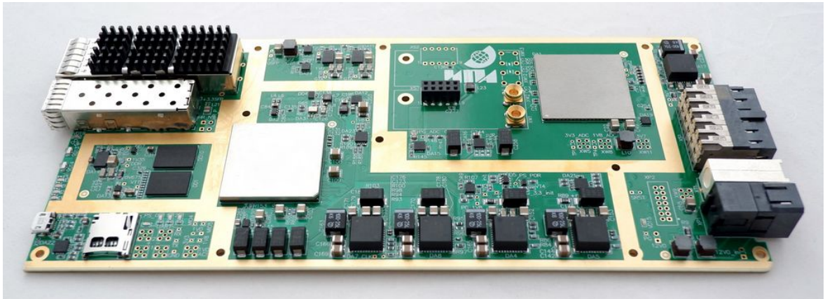
Fig. 2 DSP unit without radiator, front-end board, and front panel.
