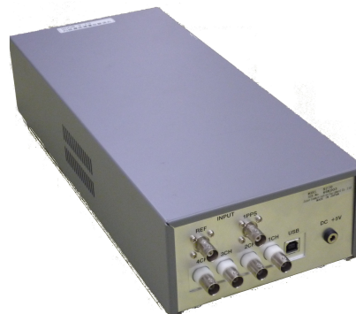
Fig. 3 One unit of the K5/VSSP32 sampler has four video signal inputs. Data output and remote control are made via a USB2.0 interface. One geodetic terminal of 16 video signals is composed of four units of this device.
