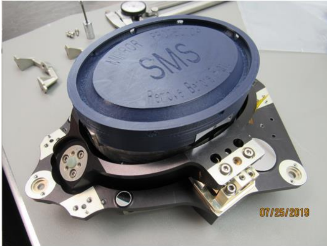
Figure 15 - L'Ralph FLT Scan Mirror Mechanism (SMM) Mirror View
