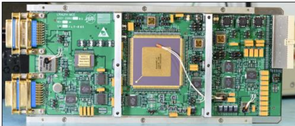
Figure 14 - L'Ralph Flight Mechanism Control Electronics (MCE)
