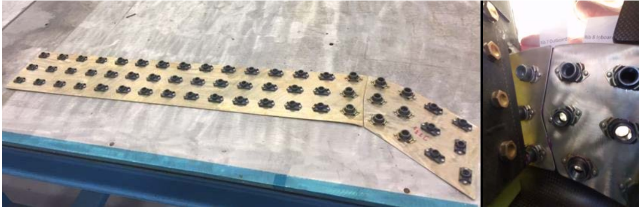
Figure 5.7. Nutplate carrier assembled (left) and installed (right).
