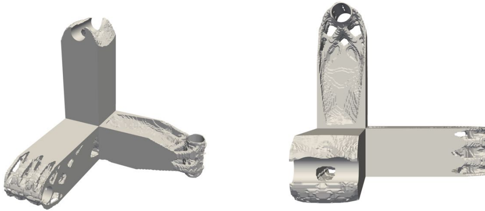
Figure 44: Isometric and top views of the mass-constrained compliance minimization result for the orthogonal bracket problem
