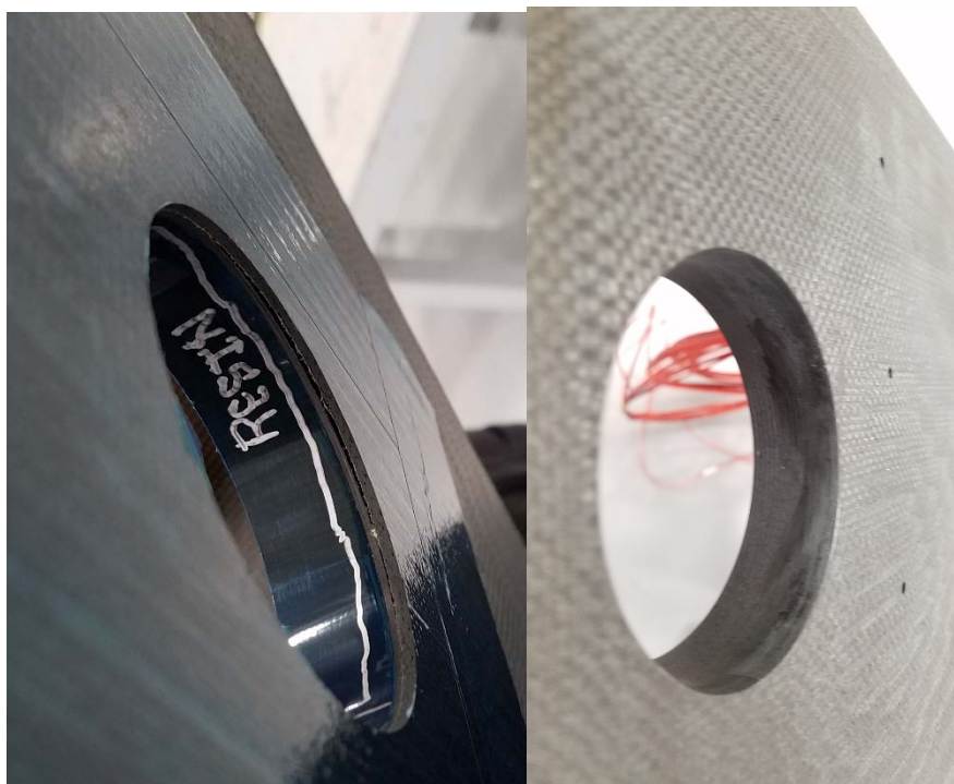
Figure 5.3. Leading edge spar web sacrificial ply delamination (left) and attempted repair (right). The repair delaminated during assembly but shim was deemed to be nonstructural.
