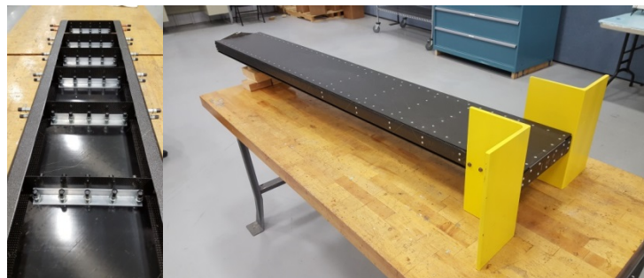
Figure 2. Hershey bar wing in fabrication, showing ribs and shear clips (left) and fully assembled (right).
