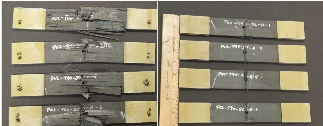
Figure B.2. Longitudinal (left) and transverse (right) OHT coupon from curvature-dominated tow-steering panels.
