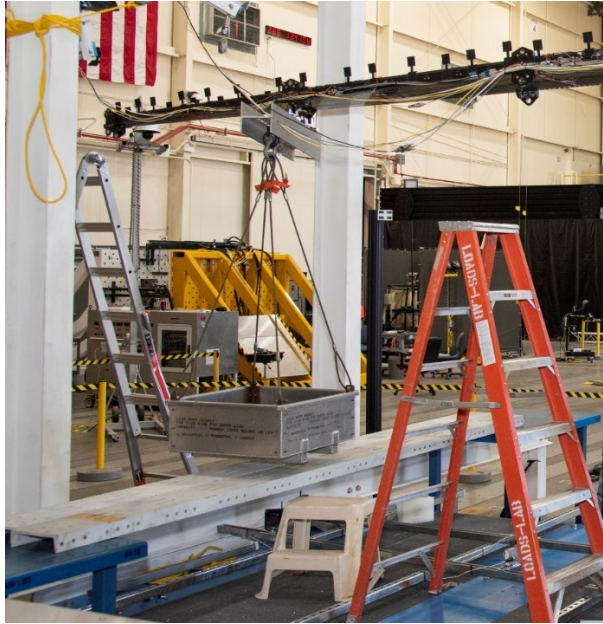
Figure 7.5. Testing hardware for 'shotbag' flexural axis testing.
