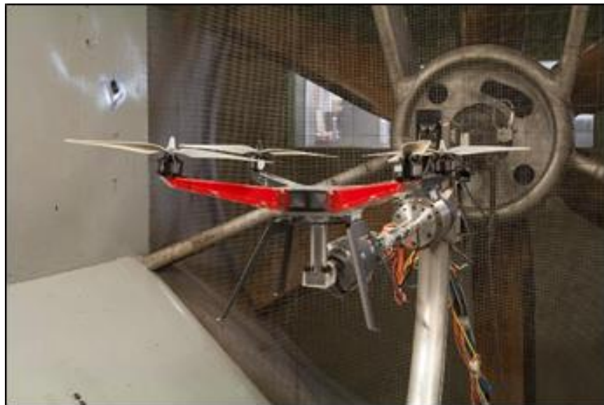
Figure D-1. Static wind tunnel testing of a small quadcopter for aerodynamic database development (NASA LaRC 12-Foot Tunnel)
