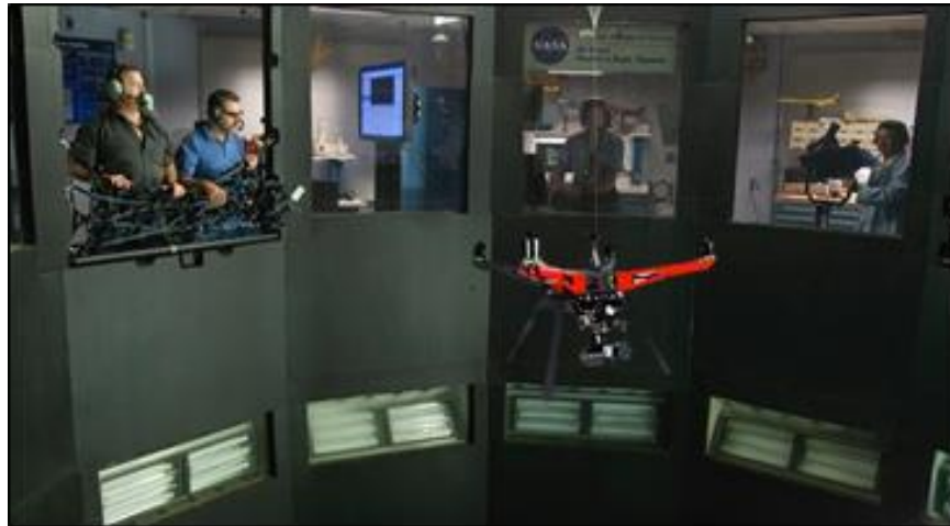
Figure D-2. Free-flight wind tunnel testing of a small quadcopter for aerodynamic database development (NASA LaRC 20-Foot Vertical Spin Tunnel)
