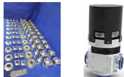
FIGURE 2. Manufacturing progress (left) and rendering (right) of Marshall dust-tolerant air selector valve.
