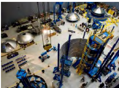
FIGURE 1. Full-scale welding of development and flight (SLS components, tanks, etc.) hardware.
