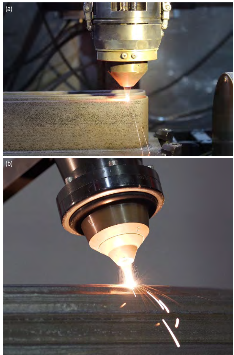
FIGURE 1. Blown powder being deposited through a nozzle onto an additive manufactured build with (a) showing a side view and (b) showing a closeup view of the nozzle exit.
