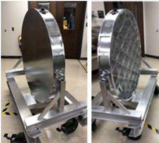
FIGURE 1. 1.2-m aluminum mirror.
