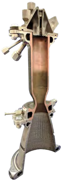
FIGURE 1. 1,200 lbf thrust subscale regen-cooled engine cut-away view showing copper-based alloy TCA, directed energy deposition nozzle, and composite overwrap.
