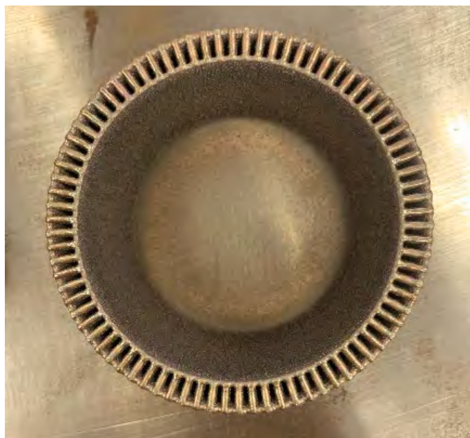
FIGURE 2. GRCop-42 channel geometry built with FormAlloy X-Series.
