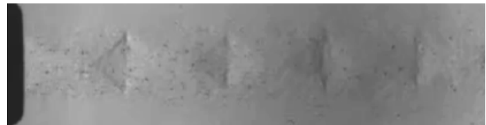
FIGURE 4. Instantaneous snapshot of particle shadows overlaid on Schlieren imaging to capture both gas flow and particle dynamics.
