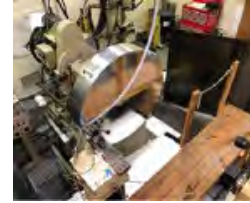
FIGURE 2. Diamond turning 1.2-m aluminum mirror.
