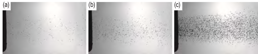
FIGURE 2. Instantaneous snapshot of particle shadow images for different mass loadings: (a) \dot{m} = 0.12 g/s; (b) \dot{m} = 0.37 g/s; (c) \dot{m} = 0.94 g/s.
