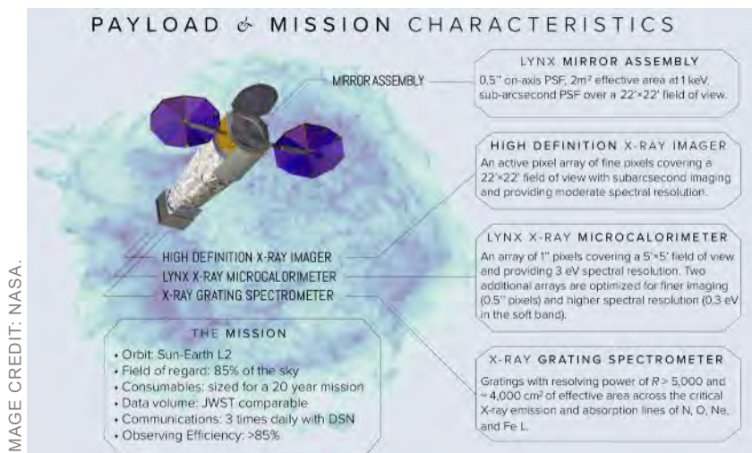
FIGURE 2. Lynx has a 10-m focal length and consists of a high-resolution, 3-m diameter, large area x-ray mirror assembly with pre- and post-collimators surrounded by the spacecraft bus and complemented by an instrument suite that includes a low-noise megapixel imaging array (HDXI); a large-format, high-spectral-resolution, small-pixel array (LXM), and high-efficiency, high-spectral-resolution, dispersive spectrometer (XGS). Detectors for all three instruments are mounted onto the ISIM.
