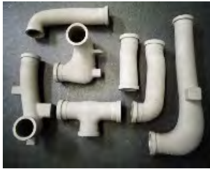
FIGURE 3. Partially finished AM air ducts with bosses and attachment tabs.
