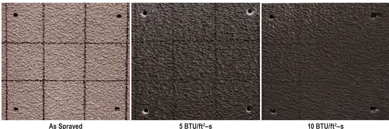
FIGURE 4. Visual comparison of TPS before and after exposure to heat.
