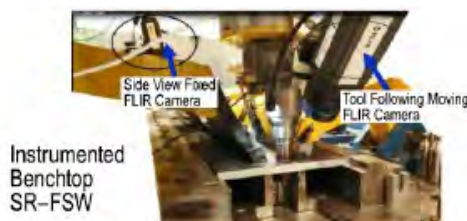
FIGURE 1. Small-scale panel level FSW welding. Typically for testing and process development.
