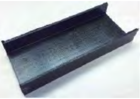
FIGURE 2. Infused and cured 36" C-channel.
