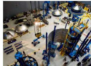
FIGURE 2. Large-scale FSW welding. From full-scale article development to flight hardware builds and welding. Pictured is MSFC’s Metal Joining and Processes Branch’s south highbay facility.
