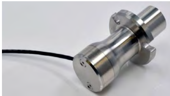
FIGURE 1. (Top) shear stress versus heat flux measurements from shear stress gauges and predictions and compared to SLS environments; (Bottom) picture of the Ahmic skin friction gauge.
