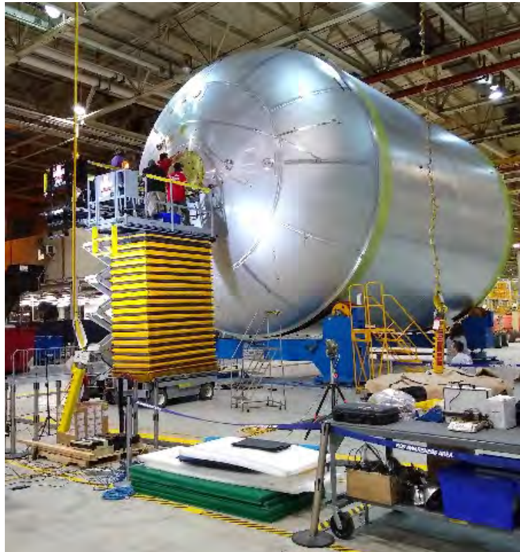
FIGURE 1. Image of the LOX forward dome during installation of the manhole cover.
