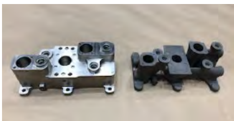
FIGURE 3. PPSA manifold traditionally manufactured (left) and additively manufactured (right), resulting in ~40% mass savings.
