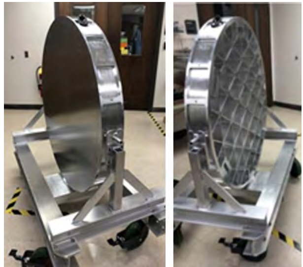
FIGURE 4. 1.2-m aluminum test mirror.
