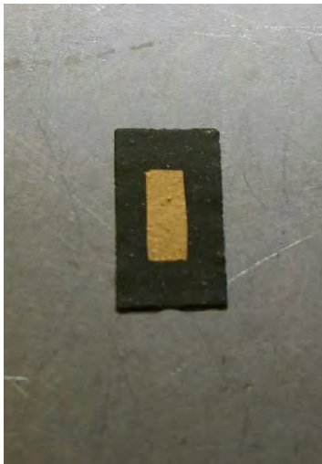
FIGURE 1. 3D-printed sensor with gold electrodes for testing piezoelectric response.
