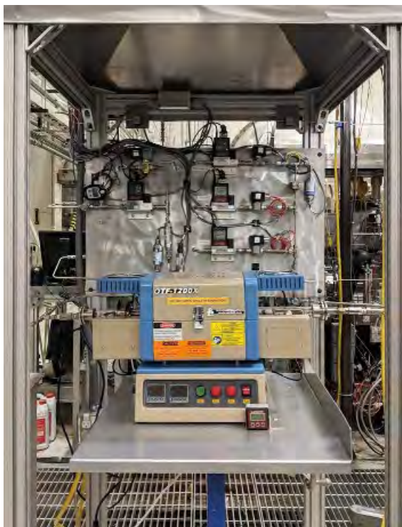
FIGURE 2. Laboratory rotary kiln reactor in rotary furnace. A custom quartz tube is used as the reactor in the furnace.
