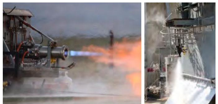
FIGURE 1B. Hot fire testing of the 5K LOX/Methane engine; and monoprop test of 3D printed engine.
