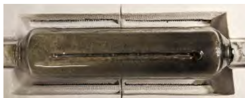
FIGURE 3. Close up of the 2 in reactor tube containing Bosch cement. In this test, carbon formation was observed to form at the location nearest the gas inlet. This indicates unbalanced flow with respect to the aspect ratio of the reactor.
