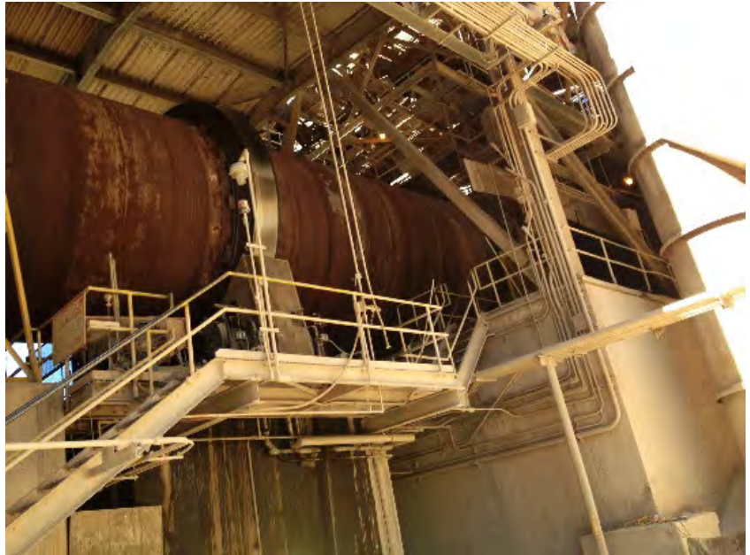
FIGURE 1. Industrial rotary kiln ( \approx 30 ft diameter) in an operational cement plant.
