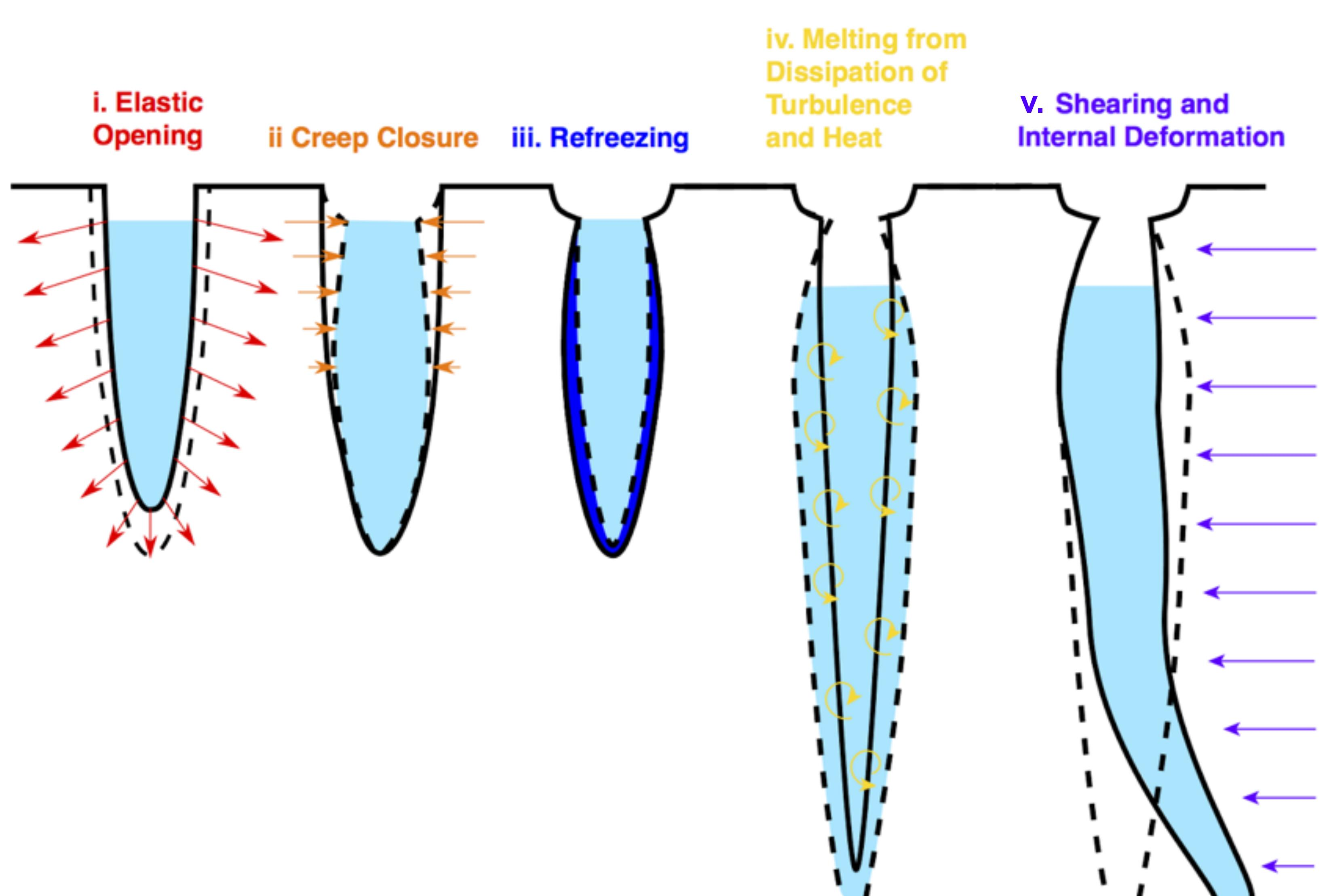
Moulin geometry evolves markedly on both short and long timescales. It may exert a first order control on the subglacial hydraulic gradient.
