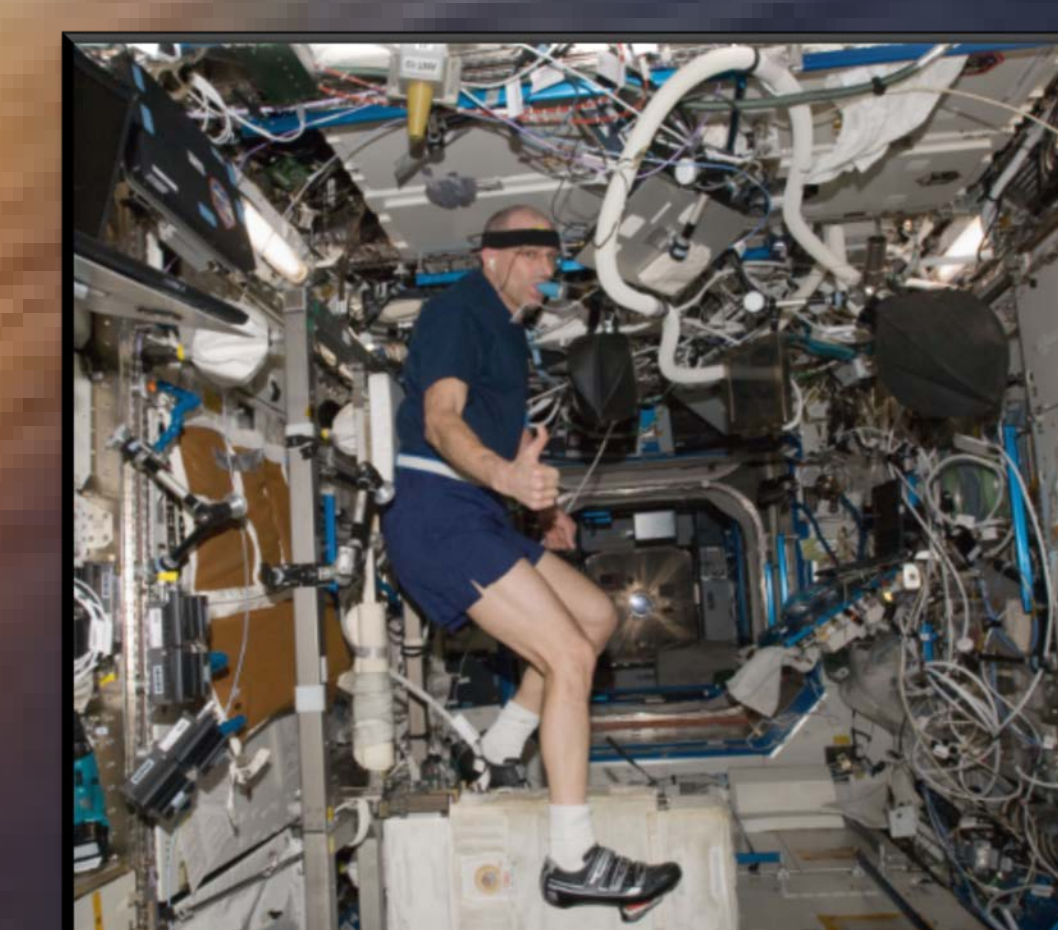
Figure 2. In-flight VO 2 pk test using the Portable Pulmonary Function System (PPFS) and CEVIS.
