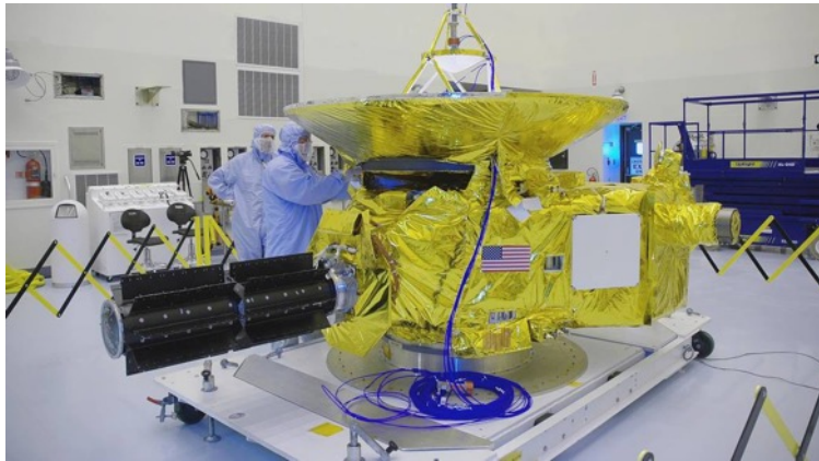
Image: RTG (left) on New Horizons spacecraft 420 W (beginning of life); mass= 57 kg (11 kg of PuO 2 fuel)
