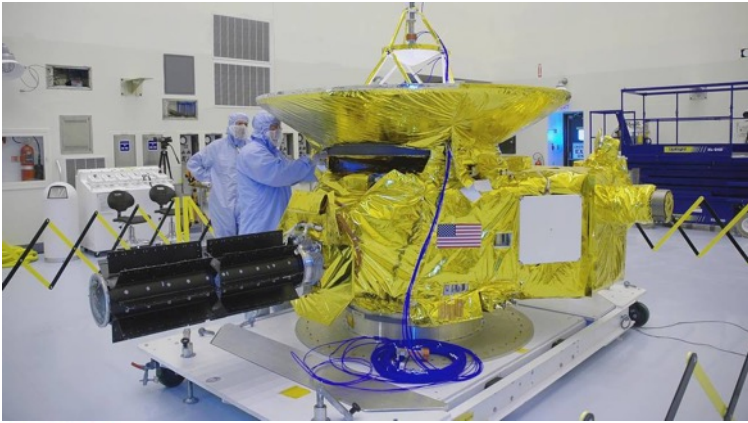
Image: RTG (left) on New Horizons spacecraft 420 W (beginning of life); mass= 57 kg (11 kg of PuO 2 fuel)
