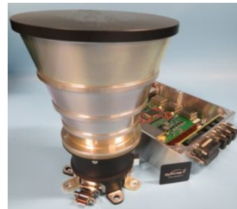
Figure 5.4: SSSL Procyon Star Tracker. Image courtesy Surrey Satellite Technology Ltd.
