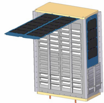
Figure 7.4: Passive Thermal Louver on 6U CubeSat Dellinger. Image Courtesy NASA Goddard (2015).
