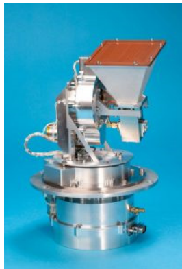
Figure 9.9: X-band high-gain antenna and pointing mechanism. Image courtesy of Surrey Space Ltd.
