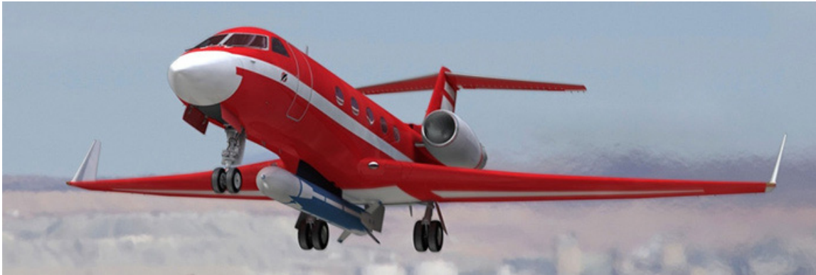
Figure 10.47: GOLauncher System mounted underneath a Gulfstream jet. Image courtesy of Generation Orbit.
