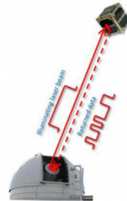
Figure 9.13: Scheme for using land-based laser to transmit data from CubeSat using on-board MRR. Image courtesy of Salas (2012).
