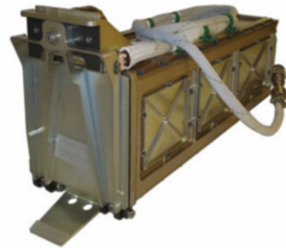
Figure 10.22: P-POD. Image courtesy of California Polytechnic State University.
