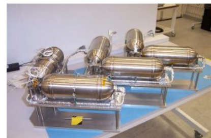
Figure 4.5: SSTL butane propulsion system. Image courtesy of Gibbon (2010).
