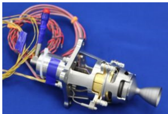
Figure 4.3: GR22 thruster. Image courtesy of Masse et al. (2015).
