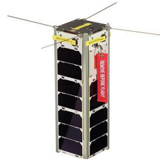
Figure 2.8: PLT3 Platform. Image courtesy of NanoAvionics.
