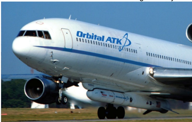
Figure 10.4: Pegasus Launch System, mounted underneath a Lockheed-1011 jet. Image courtesy of Northrop Grumman Innovation Systems.
