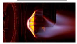
ADEPT uses novel 3d woven carbon fabric as TPS/structural membrane suitable for high thermal conditions for Venus and Mars entry
