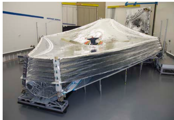
Figure 9: Left -- A 1/3 scale fully functional model of the sunshield was used for design verification in a cryo-vacuum chamber equipped with solar simulator lamps; Right -- A full scale engineering model of the sunshield.
