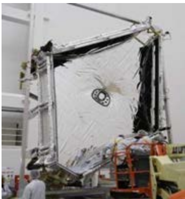
Figure 9: Left -- A 1/3 scale fully functional model of the sunshield was used for design verification in a cryo-vacuum chamber equipped with solar simulator lamps; Right -- A full scale engineering model of the sunshield.
