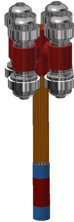
Figure 4. Welded secondary heat exchanger concept with (8) 1.5 kW e Stirling convertors arranged in a dual opposed configuration
