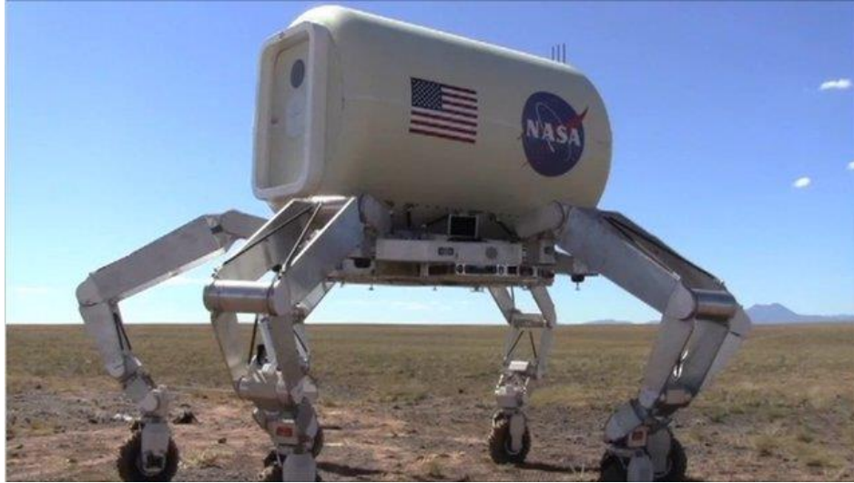
Fig. 1 Half-Scale ATHLETE Prototype Carrying Mockup Habitat Module
