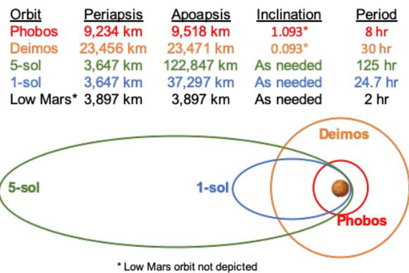
**Figure 3. Orbits of various Mars staging locations.**
