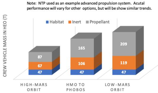
**Figure 4. Example total crew vehicle mass for various Mars orbits.**
