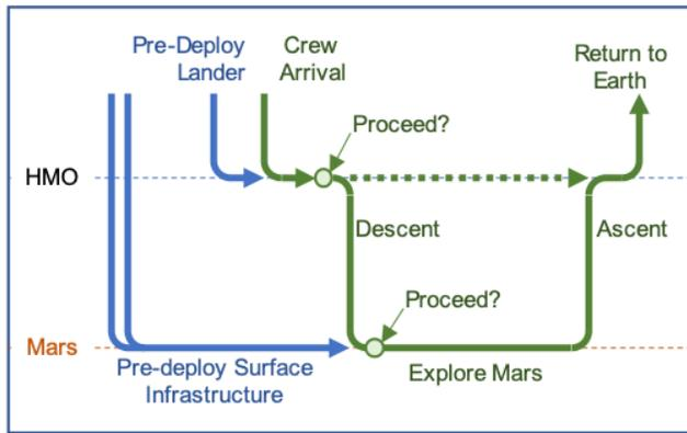
**Figure 7. Human exploration of Mars operational concept.**
