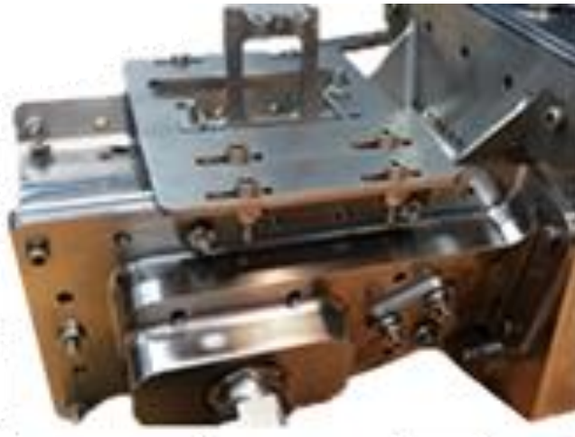
Figure 1.6b.1. Photograph of N+3 combustor hardware for NASA testing, during preliminary assembly.
