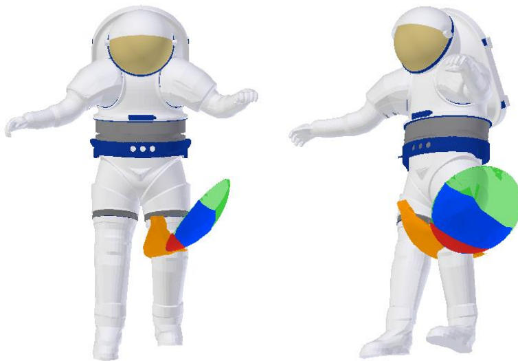
Figure 12. Mark III hip mechanical RE (green) overlaid with the RE envelope found from HITL motion capture data during functional tasks that were done unsuited (orange) and in the Mark III (blue). The red region indicates the area of overlap between the functional ROM used by the subject in the unsuited condition and the mechanical RE of the Mark III.
