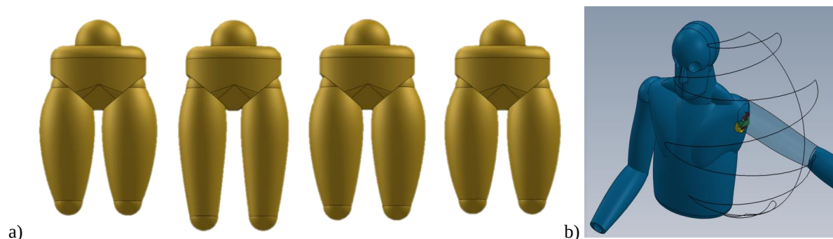
Figure 1. First iteration of “anthronaut” models representing a range of anthropometry for the lower body (a); Anthronaut subject demonstrating a prescribed reach envelope of the shoulder (b).
