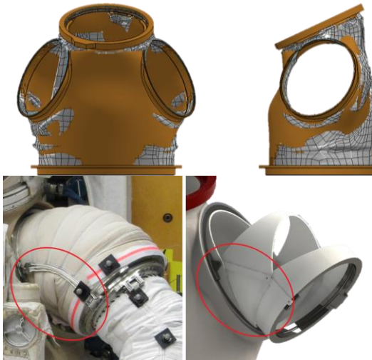
Figure 5. EMU CAD model of the upper torso hard goods (top); the comparison between the 3D scans and the modeled HUT (center), and the comparison between the actual EMU shoulder (bottom left) and modeled 3-convolute shoulder (bottom right) with the restraint line circled.
