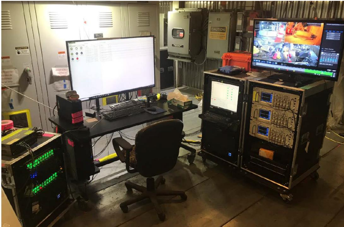
Figure 6: Test Control Center (DAQ and Shaker Monitoring System)
