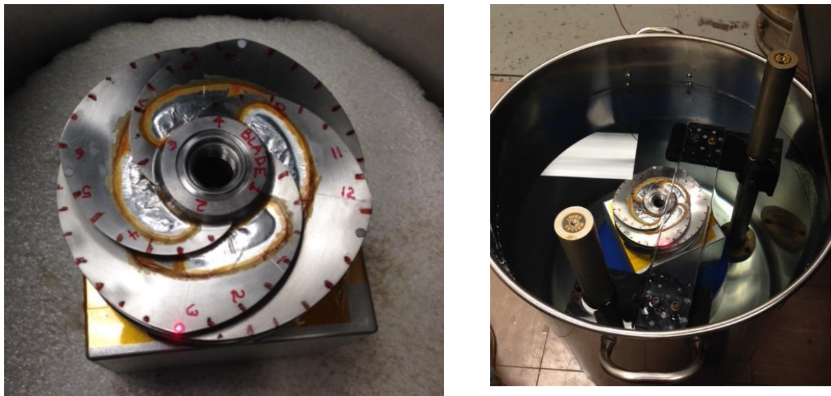
Fig. 5 Subscale Inducer Modal Test in Large Tub of Water
