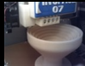
Antenna Feed Horn which is being tested with various printed coatings for in-space use Printed 3/9/17 and returned on SpaceX-10 3/20/17
