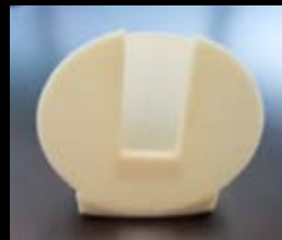
Radiation Enclosure Module (REM) printed in different thicknesses to hold monitors for radiation testing Printed 3/20/17, 5/30/17, and 6/16/17
