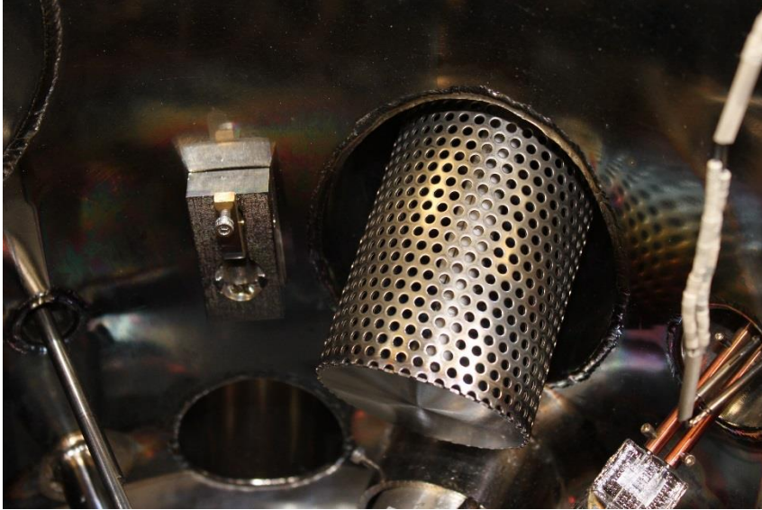
Oxygen Pump inside the levitation chamber.
