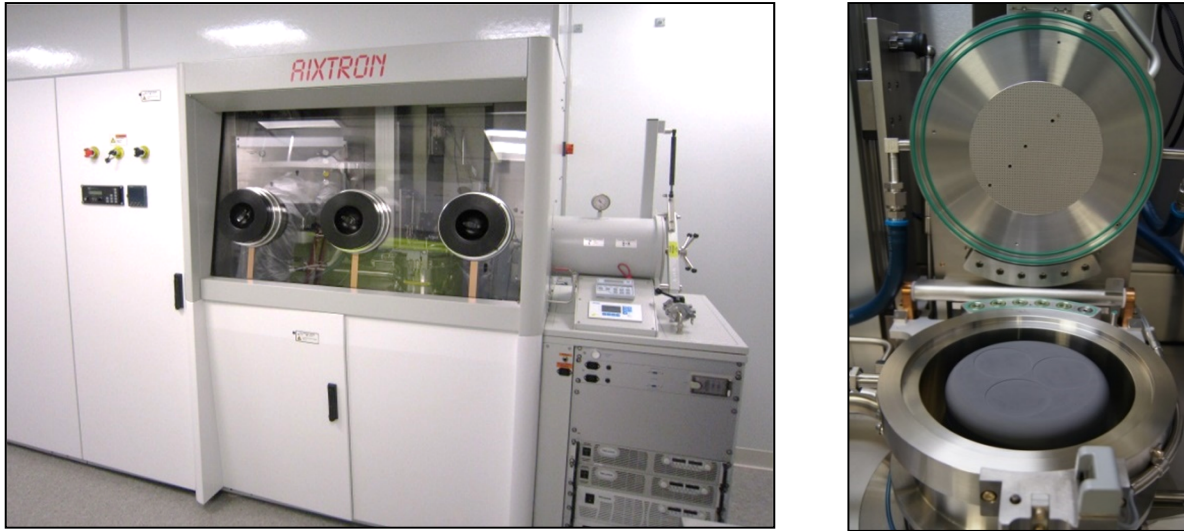
Figure 1. High-temperature MOCVD system with close-coupled showerhead for UV-APD development [5].
