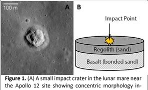
the Apollo 12 site showing concentric morphology inferred to be a result of a layer of regolith over a more competent unit [-3.297°S/336.708°E] (B) Layered target design. Stronger substrate of bonded sand underlies a thin layer of loose sand ("regolith").
