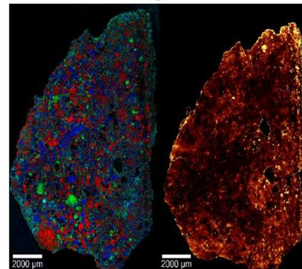
Figure 1: Image on the left shows the Raman mineral maps of pyroxene, olivine, and multi-molecular carbon (MMC) within ALHA-78085 prior to incubation with *F. oxysporum*. Image on the right depicts an attempt at determining the fungal coverage after incubation; however, the wavelength used to locate fungal coverage was extremely similar to one type of background fluorescence.
