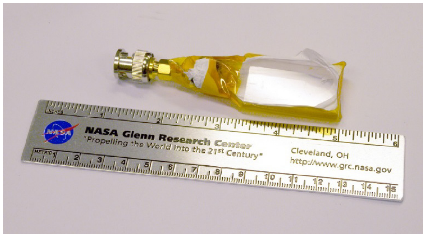
Figure 17.—Miniature scintillation-diode ionizing radiation detector as demonstrated (Wrbanek and Wrbanek, 2016).
