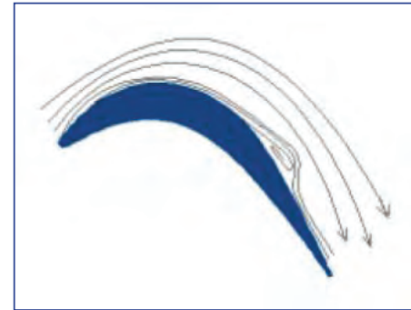
High-load LPT blade at low-Re
