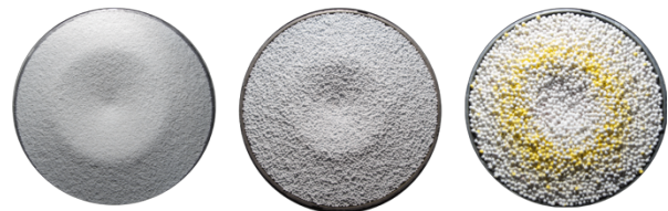
Figure 1. Photos of impact craters formed in coarse targets at the AVGR. From left to right: 2 mm, 6 mm, and 12 mm diameter alumina spheres. Crater morphology becomes increasingly irregular as target grain size increases, even for these hypervelocity impacts at \sim 5 km/s (The pre-impact surface of the 12 mm spheres was painted yellow to make the final crater more obvious.) The target bucket is \sim 60 cm across.
