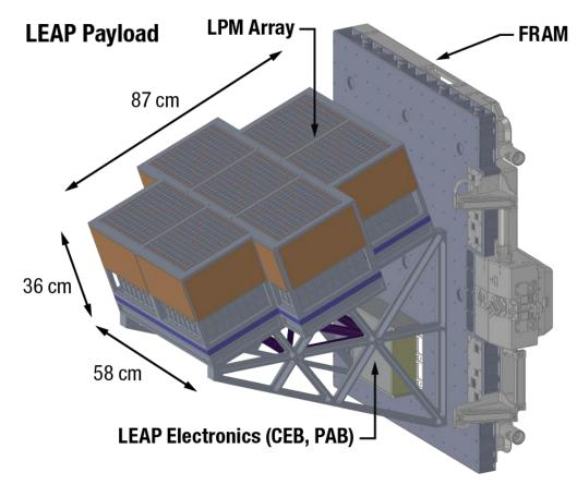
Full LEAP instrument consists of 7 independent polarimeter modules surrounded by passive Pb shielding on sides and bottom.
