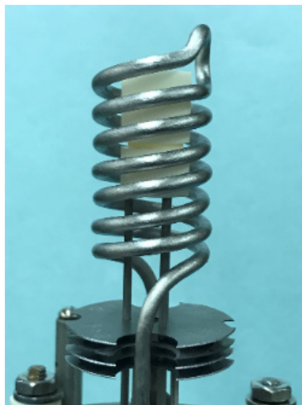
Figure 5.—Tantalum helical elemental around an alumina Knudsen cell.
