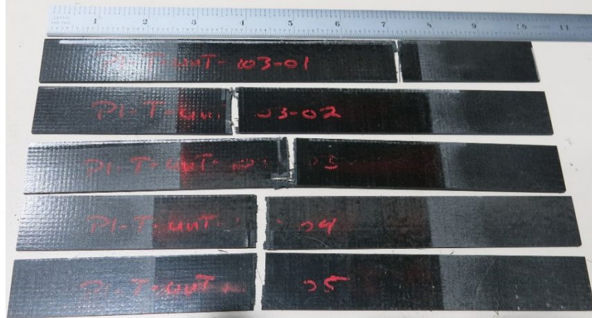
Figure 3.—Failed IM7/8552 Samples Subjected to Longitudinal Tension.
