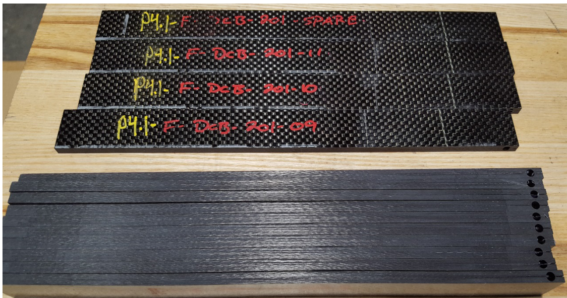
Figure 31.—Example of Prepared DCB Specimens with Loading Holes.
