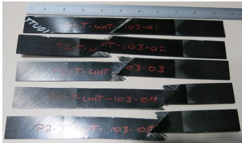
Figure 7.—Failed IM7/8552 Samples Subjected to In-Plane Shear.
