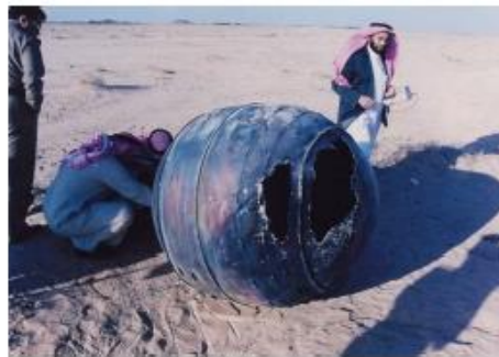
Titanium casting of STAR-48B SRM (Saudi Arabia, 2001)
