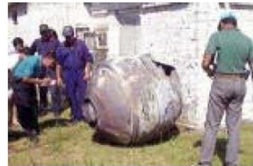
Titanium casting of STAR-48B SRM (Argentina, 2004)
